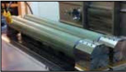
Figure 1. Dual magnetron sputtering arrangement, with rotatable magnetrons
