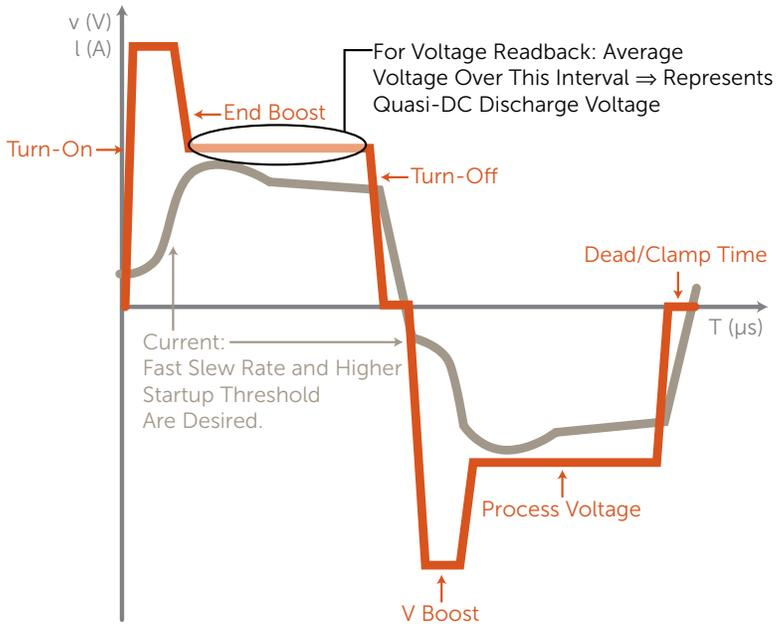
Figure 3. Baseline output waveform, showing region for sputtering voltage measurement
