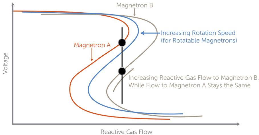
Figure 2. Voltage versus reactive gas flow control space of a dual magnetron system
